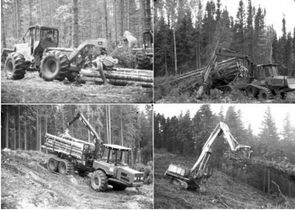
Fig. 10.2 Ground-based equipment travels to the stump and brings logs/trees back to the landing. A wheeled or tracked grapple skidder (top left) can quickly grab bunches created by a feller-buncher, although a cable winch with chokers can replace the grapple in manually felled timber. A clam-bunk skidder (top right) can assemble and skid a much larger turn. A forwarder (bottom left) can collect a large turn from logs that have been felled and processed by a harvester. A shovel or log loader (bottom right) swings trees/logs towards the landing.
