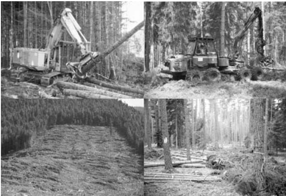
Fig. 10.1 A feller-buncher (top left) fells trees into bunches (bottom left). A harvester (top right) fells and then delimits and bucks the trees in its path, creating a slash mat that protects the soil. Logs are dropped in bundles or bunches to both sides of the yarding corridor (bottom right).
