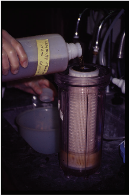
FIGURE 17.9 (A) Field Viradel system for concentrating viruses from water. (B) Elution of virus from filter with beef extract. (Reprinted from Environmental Microbiology © 2000, Academic Press, San Diego.)
