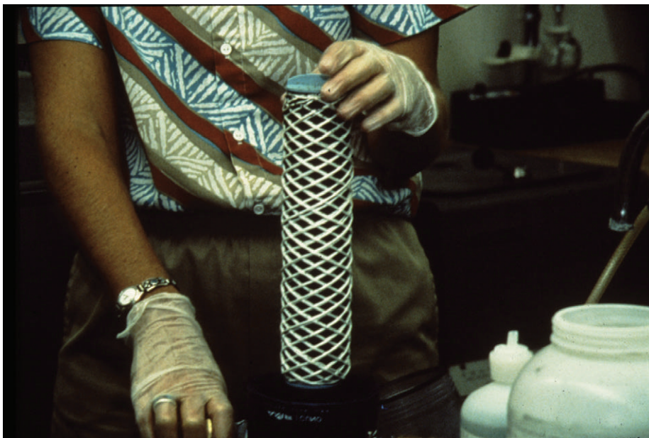
FIGURE 17.14 Spun fiber filter for concentrating Giardia cysts and Cryptosporidium oocysts. (Reprinted from Environmental Microbiology © 2000, Academic Press, San Diego.)
