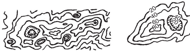
FIGURE 5.6 Enclosed depressions (e.g., sink holes, kettles) are shown by hachure lines on contours. Hachures point towards the center of the depression.
