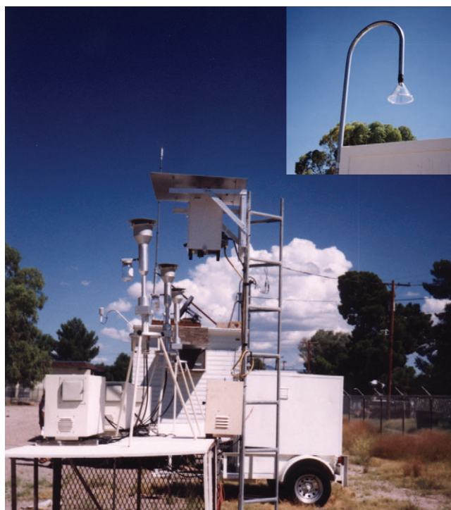
FIGURE 10.10 An air quality monitoring station near a residential area in Tucson, Arizona. Meteorological sensors and particulate matter samplers are visible in photograph. Note the air sampling probe ( insert ) through which air is drawn to analytical instruments inside the trailer. (From A. Matthias.)
