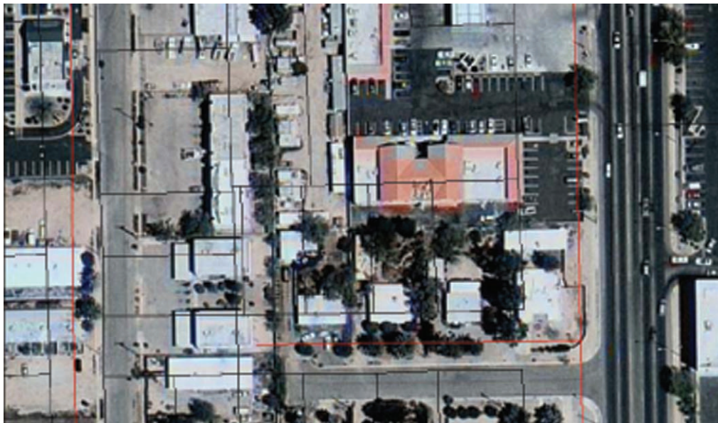
FIGURE 6.5 Orthophoto of Tucson, Arizona. Note that the parcel boundaries do not match up to the lots and will need to be corrected with “rubber-sheeting.”
