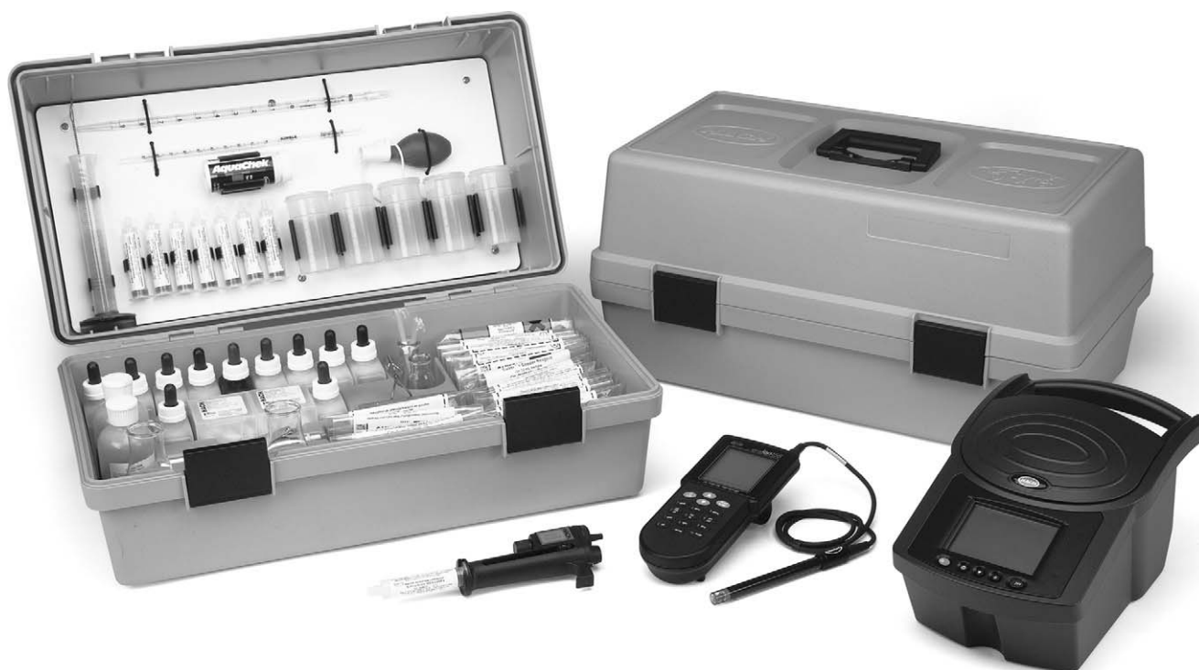
FIGURE 9.12 Field portable water quality kit. It includes one or more portable colorimeters, premeasured reagents, and step-by-step operating instructions for the analysis of multiple water quality parameters in the field. (Hach Company Catalog, P.O. Box 608, Loveland, CO 80539-0608.)
