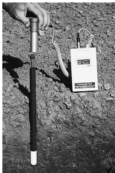
FIGURE 12.25 Tensiometer and tensimeter. (Courtesy Soil Measurement Systems, Inc. Tucson, Ariz.)
