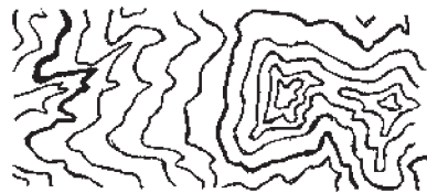
FIGURE 5.5 Contour lines are shown on most topographic maps as brown lines. Heavier lines (every fifth contour) are used to designate major units of elevation.
