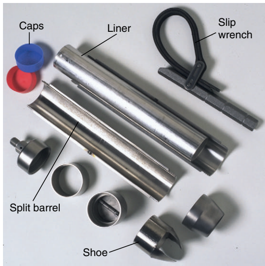
FIGURE 7.7 (A) Shelby tube, comprising a single piece, thin-gauge metal tube with a sharpened point. Sampler head connects tube to extension rod for manual or power sampling. Ball valve releases air during sampling. Ends are capped following sampling, and the tube is stored in an ice cooler for laboratory analyses of sample. (B) Split spoon sampler. (A, After Foremost Mobile Co., Inc. B, (From Ben Meadows Company, a division of Lab Safety Supply, Inc.)
