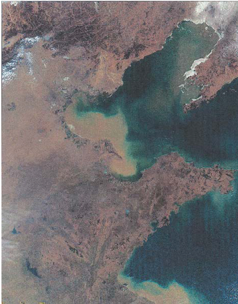
FIGURE 11.14 MODIS image showing sediment transport at the mouth of the Yellow River on February 28, 2000. Soil erosion from the Loess Plateau is proceeding at a very high rate. (Courtesy Jacques Descloitres, MODIS Land Rapid Response Team, NASA/GSFC.)
