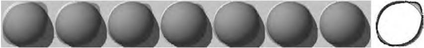
Fig. 18.1 Iterative correction of positional inaccuracies of an ellipsoid mapping unit to an artificial hemisphere DEM. The left image is the original ellipsoid followed by images showing the results after 2, 4, 6, 8, 10 and 12 iterations. The image in the right shows the location of the corrected pixels
