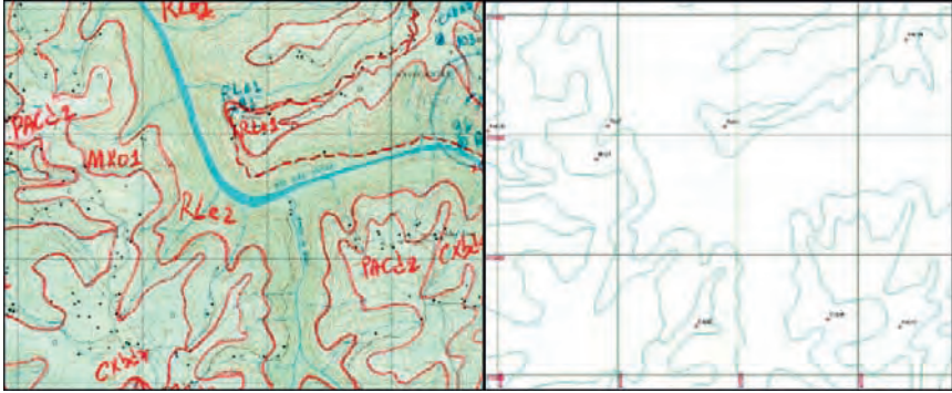
Fig. 9.3 The topographic map sheet resulting from the field work and the mapping units after digitized (See also Plate 10 in the Colour Plate Section)
