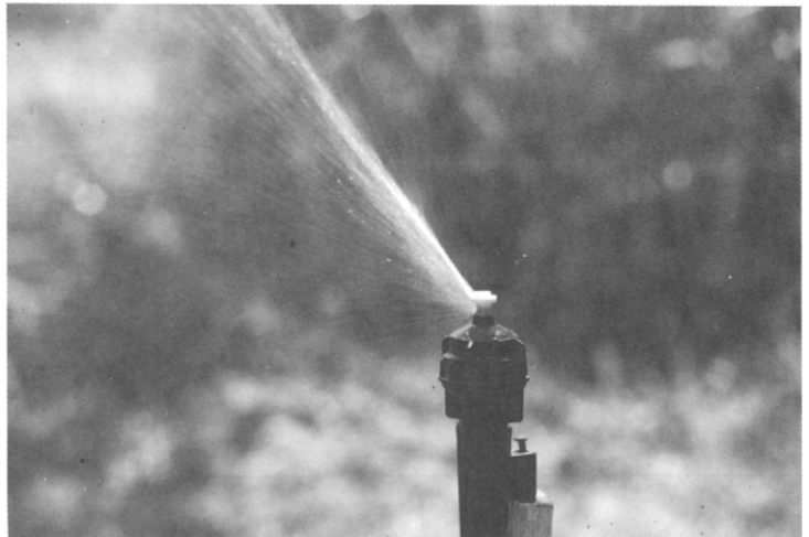
Figure 7.6 Minisprinklers have moving parts to spread water over a larger wetted area whilst maintaining reasonably low operating pressure.
