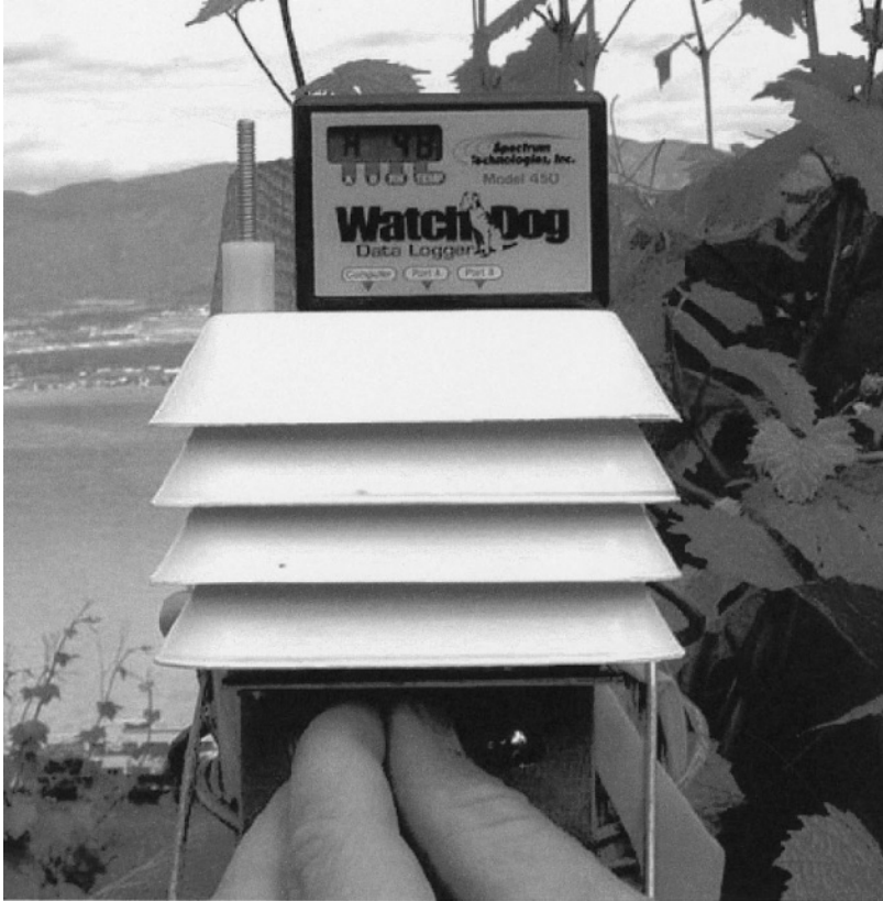
Figure 2: Miniature weather station in a vineyard in British Columbia, Canada. The Watch Dog datalogger has been removed from its protective weather enclosure so it can be seen. This particular datalogger records leaf wetness, relative humidity, and temperature for use in forecasting powdery mildew.
