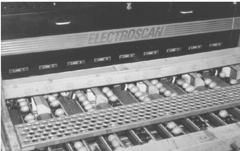
Figure 10: Electronic grader for grading size, shape, colour and blemishes of fruit
