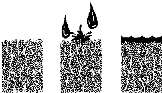
Fig:31. Sealing of the Soil Surface by Raindrops
