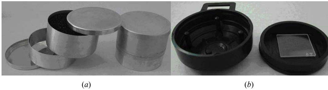
Figure 20. Measurement devices for indoor ^{222}\text{Rn} activity concentration: (a) activated charcoal collector and (b) diffusion chamber with SSNTD.
