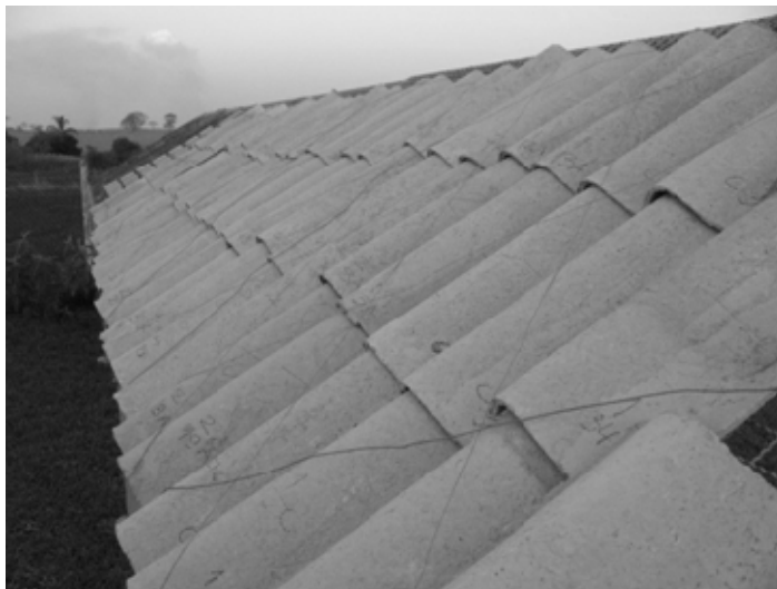
Figure 18. Roofing tiles exposed to natural ageing in Brazil.
