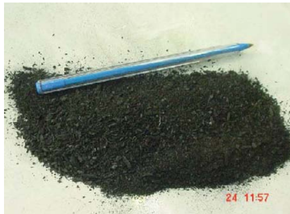
Figure 4. Biochar produced from agricultural waste through pyrolysis process (Photo: Best Energies Australia).
