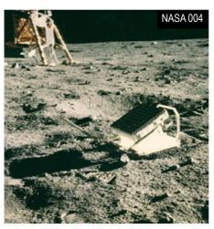
Apollo 11 Landing Module (picture corner) and the Laser Ranging Retro-reflector Array. The reflector was left by Apollo 11 crew on the landing site, and is still used today by the McDonald Observatory to monitor the precise Earth-Moon distance. (http://www.csr.utexas.edu/mlrs/)
