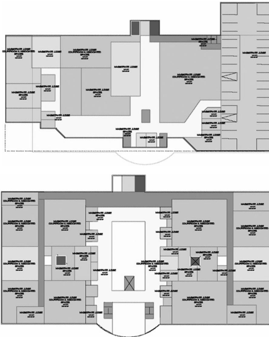
FIGURE 5-7 Example BIM model of a preliminary concept design for a two storey courthouse.
