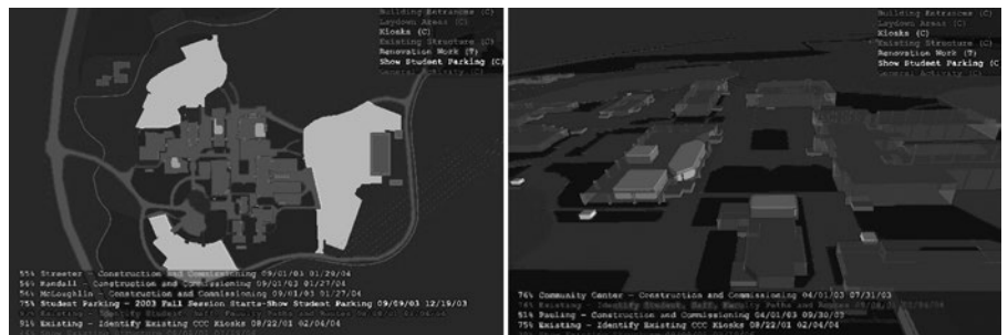
FIGURE 6-12 4D snapshots of a campus-wide project showing various construction activities occurring throughout the campus to landscape, road, and facilities.
