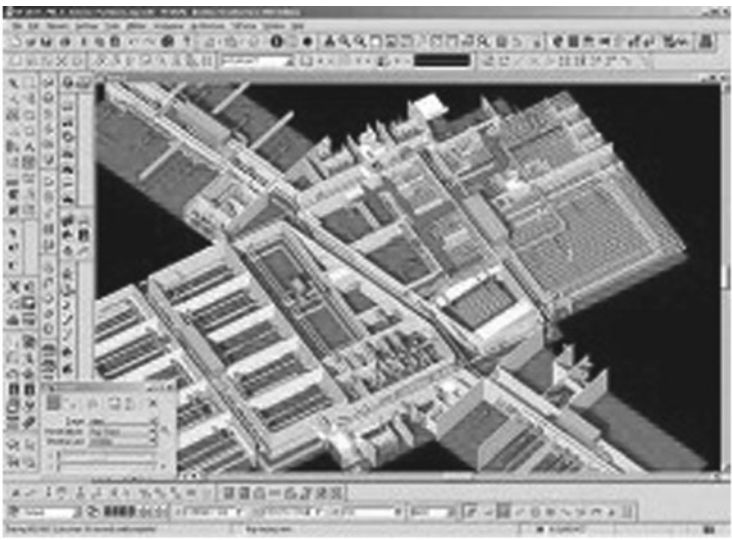
FIGURE 4-4 Example of BIM space modeling by Jacobs Facilities, where they used spatial information to check the design against program requirements and to evaluate such things as natural lighting and energy efficiencies during the conceptual design process.
