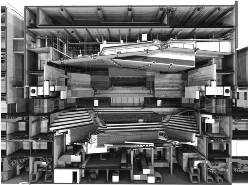
FIGURE 9-8-13 Combined model for layout and clash detection.
