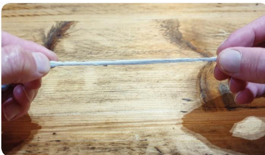
▲ When this putty is stretched, it becomes long and thin. This behavior is described as ductile
