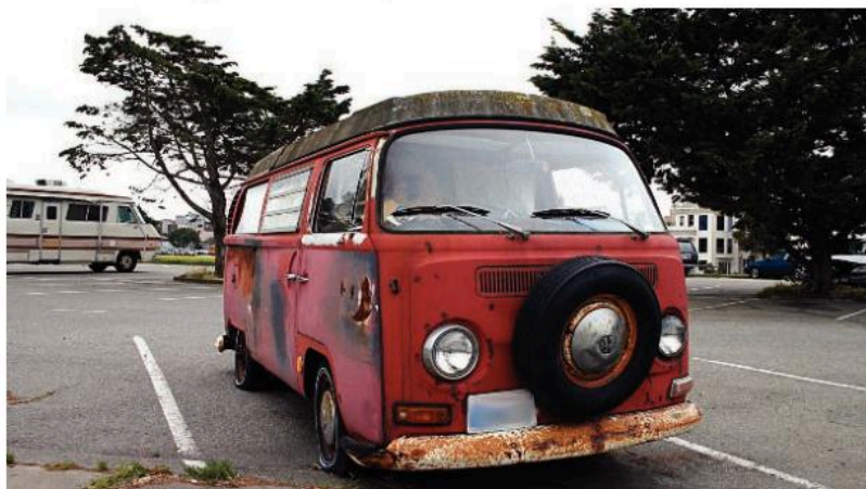
Objects containing iron will rust with water and oxygen, unless the iron is specially treated or the surface is protected.
