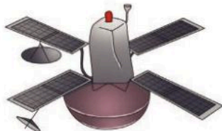
A Viking space probe, 1976, which orbited and landed on Mars to photograph, and test samples
