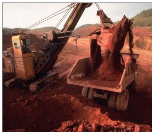
The top layers of soil and rock are removed. The bauxite is then taken out and loaded onto trucks
