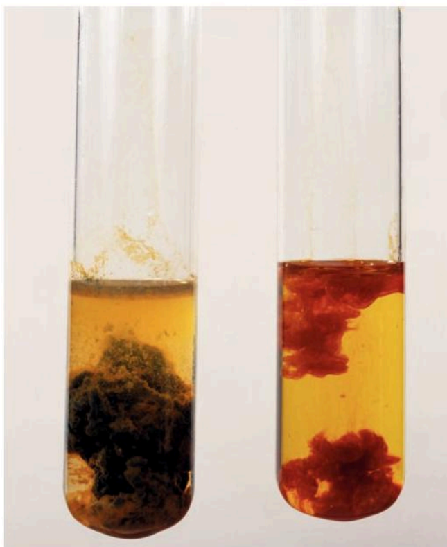
Precipitates of iron(II) hydroxide and iron(III) hydroxide
