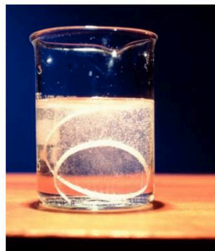
Magnesium reacting with dilute sulfuric acid
