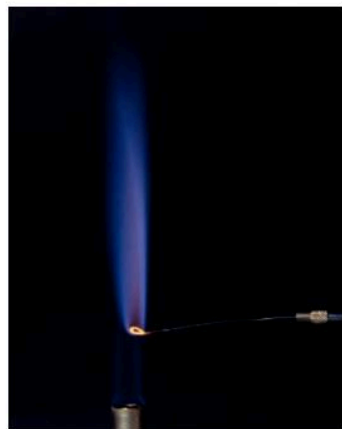
The flame test for potassium
