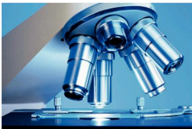
This microscope has a wide range of objective lenses so that different magnifications can be used
