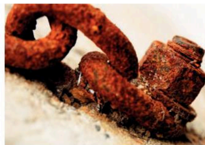
Rust flakes away easily exposing fresh iron to air and water
