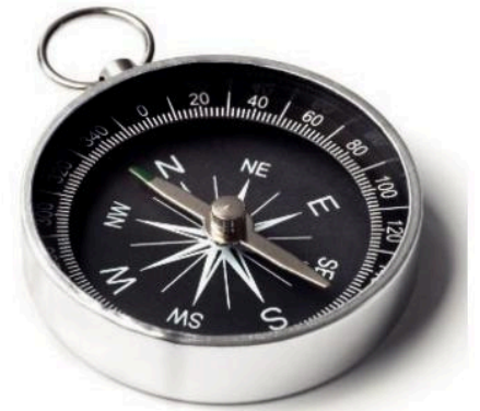
The north pole of a compass will always point in the direction of the magnetic field
