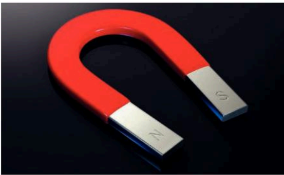
Magnets can be shaped into U or horseshoe shapes to bring the poles closer together. This makes the magnet much stronger
