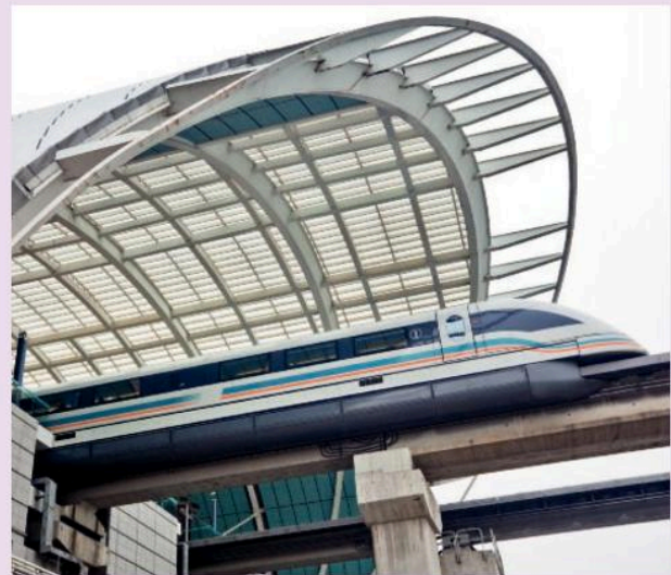
This train in Shanghai uses magnetic levitation – it travels smoothly at over 430 km/h
