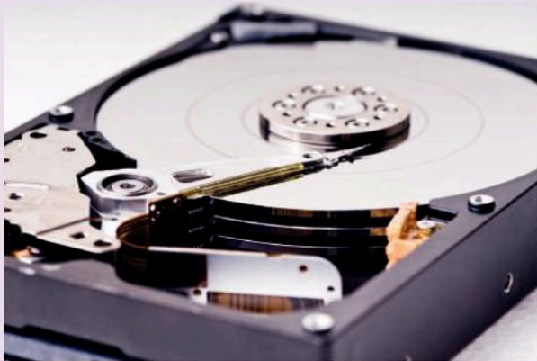
The surface of a hard disk is coated in magnetic materials
