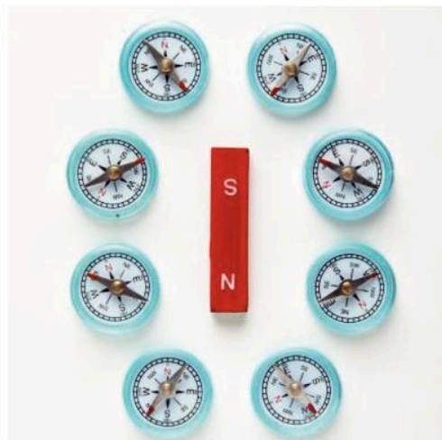
The shape of the magnetic field around a magnet is shown by these compasses
