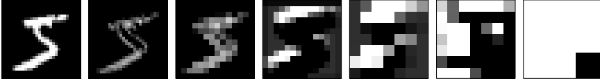
FIGURE 9.6: An image representing a handwritten digit followed by partial outputs of the layers of a convolutional neural net trained to identify digit images. Each layer output consists of a stack of two-dimensional arrays, and this figure shows only one of them per layer.
