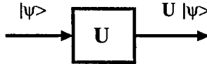
Figure 8. The diagram representing the action of a unitary matrix U corresponding to a quantum gate on a qubit in a state |\psi\rangle .
