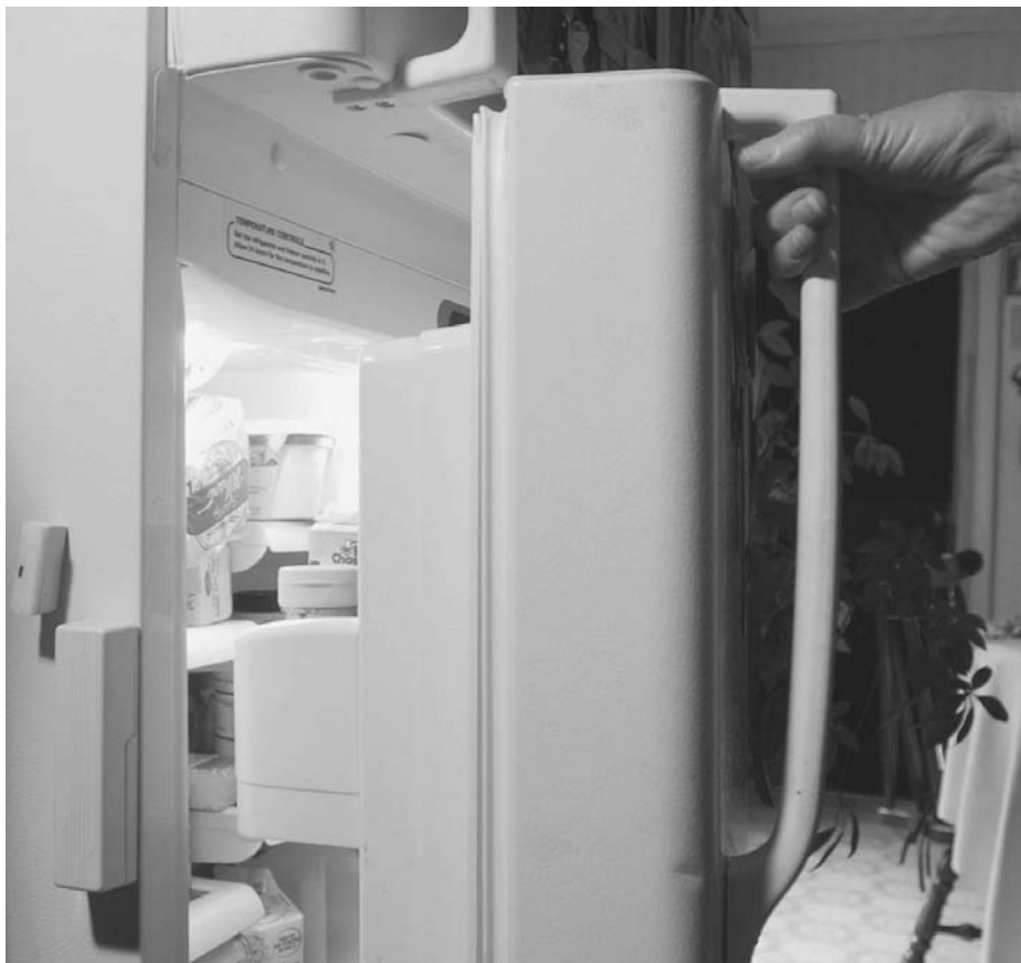
Assistive Elderly Care. A sensor on the left side of the refrigerator records and relays the opening and closing of the door. The refrigerator is monitored from a secure Internet site to make certain that senior citizens are getting food on a regular basis. AP IMAGES.
