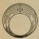
When the water at A moves toward B, the water at C, which is contiguous to A, takes its place (per Prop. 8); then from B an equal quantity must replace that at C. (per eandem). Therefore (per Ax. 14), it will move four times as fast. Q. E. D.
