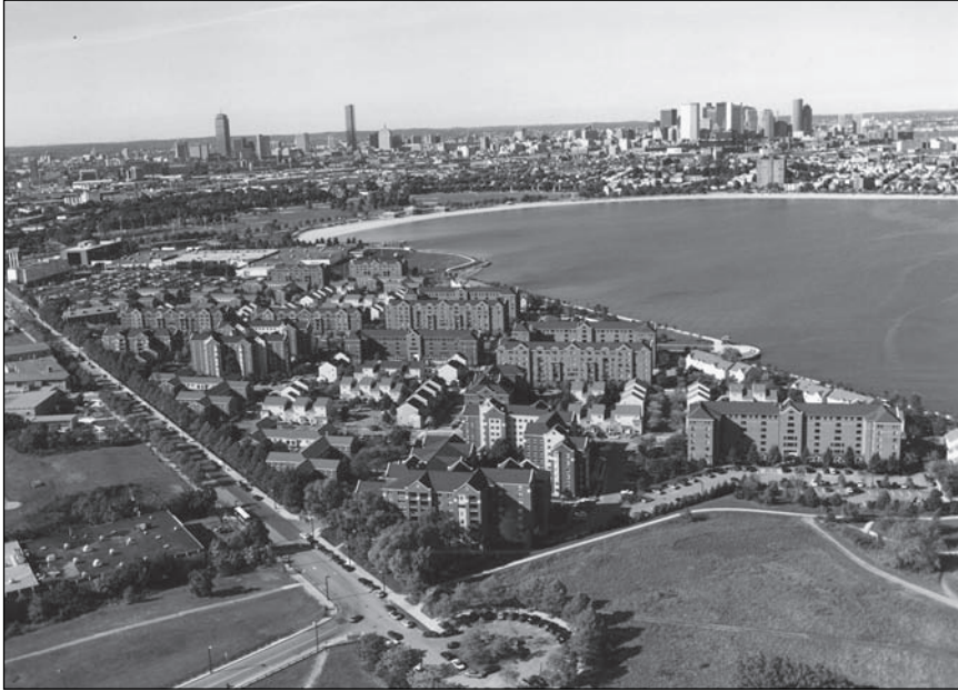
The new urbanism design of Harbor Point, which replaced Columbia Point, was modeled after thriving Boston neighborhoods, such as Back Bay. Mixed building types are set close together along narrow streets canted at a 45-degree angle to the water's edge, which opens views of the harbor and Boston skyline to all residents.
