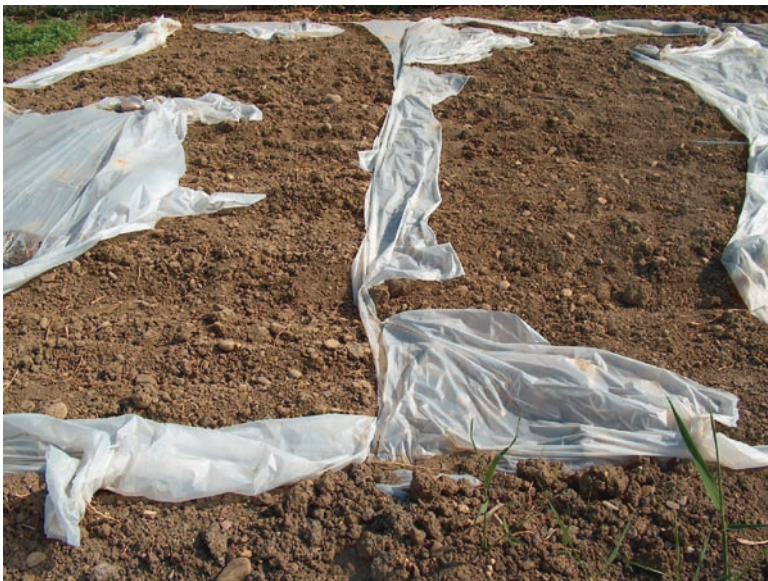
Fig. 9.3 Degradation of a biodegradable plastic film after soil solarization in a field experiment in Southern Italy (courtesy of dr Donato Castronuovo)
