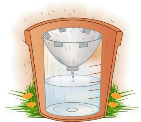
▲ Figure 2.5.9 Rain gauge
