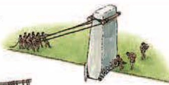
The pit around the base was packed tightly with stones and chalk.
