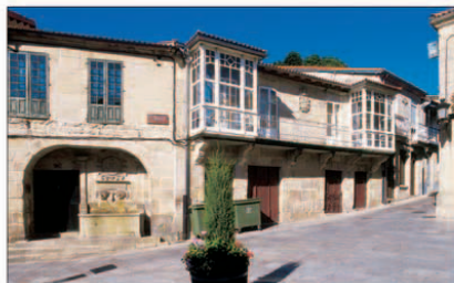
These narrow two-storey houses with glass-enclosed balconies are common in fishing villages. Their functional plan creates living space on the upper floor, with storage for fishing equipment on the ground floor.
