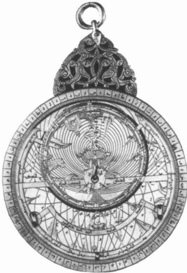
FIG. 2.16. A UNIQUE ASTROLABE, WHICH IS ALSO A MECHANICAL, GEARED CALENDAR (FRONT). This astrolabe was made in 618/1221–22 in Isfahan by Muḥammad ibn Abī Bakr al-Rashīdī. Diameter of the original: 18.5 cm. Museum of the History of Science, Lewis Evans Collection, Oxford (inv. no. IC5). By permission of the Bettman Archive, New York.
