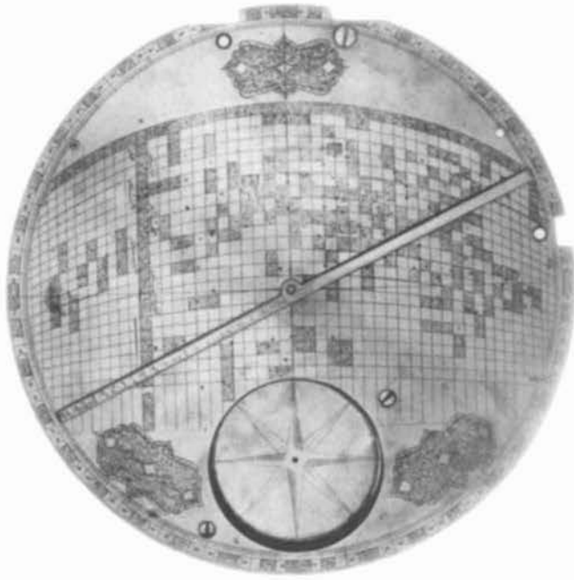
FIG. 9.16. RECT-AZIMUTHAL QIBLA MAP. This was used for finding the qibla of any locality. Mecca is at the center, and numerous cities between Spain and China, Europe and the Yemen are marked on a cartographic grid. The rule attached at the center enables one to read off the qibla on the circular scale around the circumference of the instrument, and the scale on the rule gives the corresponding distance between the two localities. This instrument came to the attention of scholars only in 1988. Diameter of the original: 22.5 cm. Photograph reproduced courtesy of the owner.
