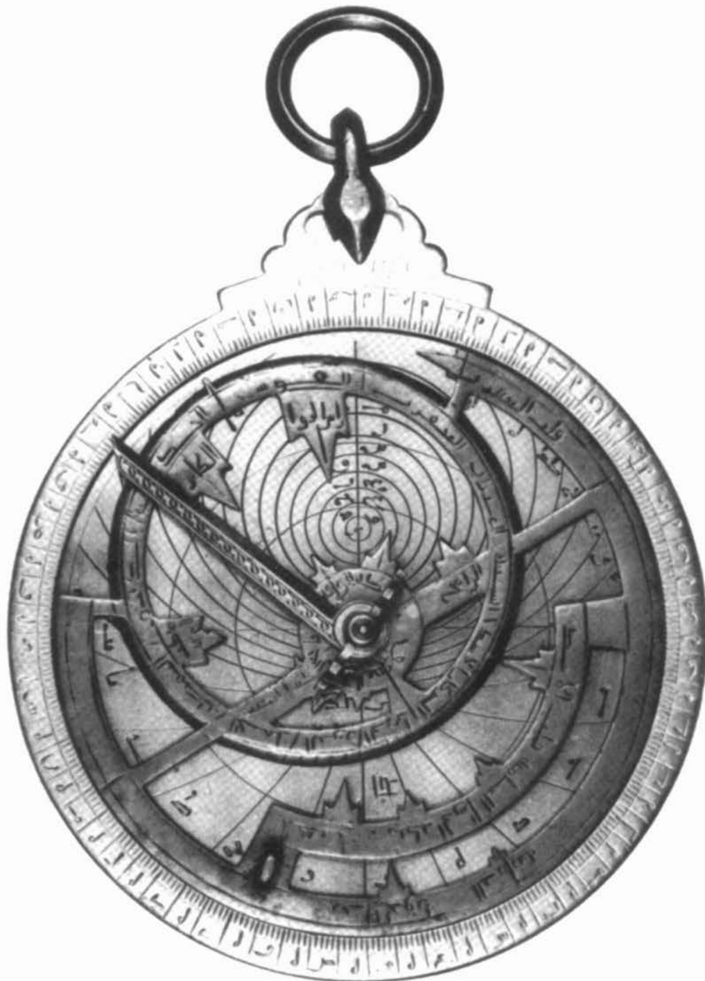
FIG. 2.5. PLANISPHERIC ASTROLABE MADE IN THE LATE NINTH CENTURY A.D. BY KHAFĪF, THE APPRENTICE OF 'ALĪ IBN 'ĪSĀ. An inscription on the front states that it was made for Aḥmad al-munajjim al-Sinjārī (Aḥmad the astronomer of Sinjār). It is known that 'Alī ibn 'Īsā, the master astrolabe maker, at the orders of the caliph al-Ma'mūn, took
