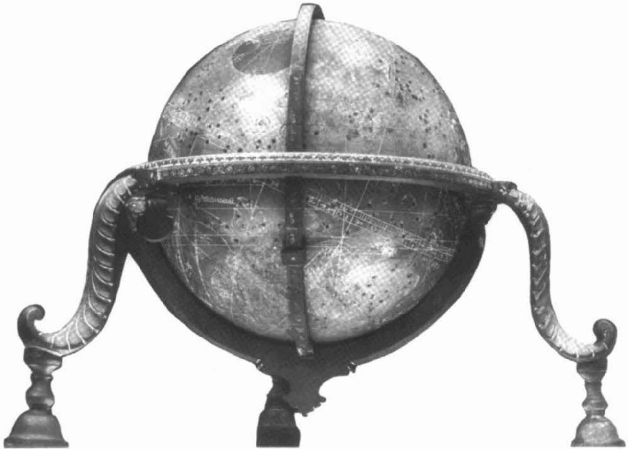
FIG. 2.31. ISLAMIC CELESTIAL GLOBE, UNSIGNED AND UNDATED, ENGRAVED IN SANSKRIT, DEVANAGARI SCRIPT. The sphere is a hollow seamless sphere cast by cire perdue . It is a product of the workshop of Lālah Balhūmal Lāhūrī, who was active in Lahore in the first half of the nineteenth century.
