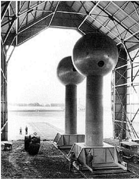
In 1931, the large Van de Graaff generator was constructed in an unused dirigible dock at Round Hill, Massachusetts. Photos © MIT.
