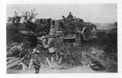
Although taken in 1918, this picture of the Gun-Carrier Darlington is typical. It shows the 6 in. howitzer in its cradle at the front, between the driver's and commander's cabs. The gun wheels are slung at the sides and extra ammunition stowed everywhere.
