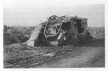
A knocked-out Mark IV on the Poelcapelle road. Only heavy artillery is likely to have caused such damage, and it could just as easily have come from a British barrage.
