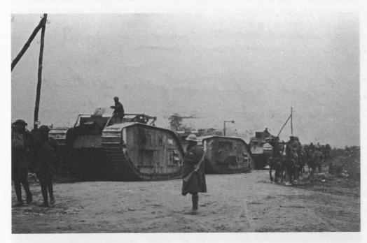
Mark V\* tanks working with the Australian Corps move through Roussay. The second tank, a male, has its semaphore-signalling device in operation.
