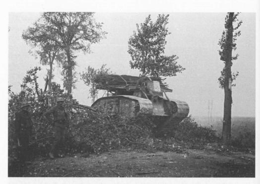
A female tank, fitted with the wider tracks, makes short work of a roadblock near Bayonvillers. It is carrying a small fascine and parts of a trench bridge.
