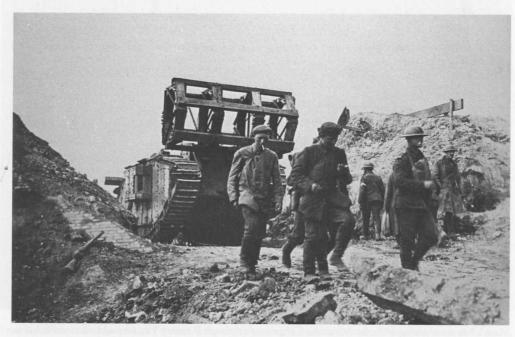
A Mark IV female tank carrying a crib, seen near Moeuvres on 27 September 1918.
