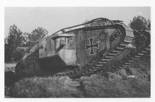
A Mark IV male tank, captured by the Germans after Cambrai and fitted with their version of the six-pounder gun.
