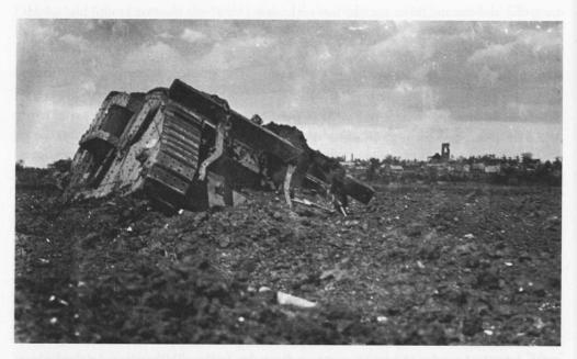
A severely ditched Mark IV female with the unditching beam still in place. If the tank was still functioning, and the crew alive, this beam would be attached to the tracks and used to lever the tank out of its predicament.
