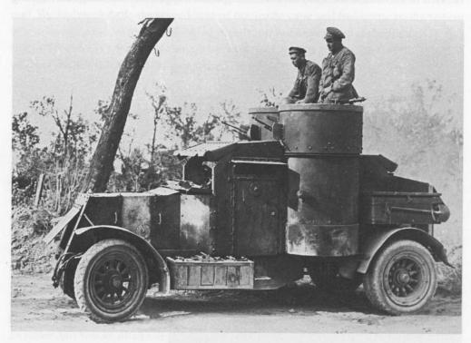
An Austin ready for action. The driver's cab is opened up, as is the radiator cover. Although they hardly compared with the Rolls-Royces used elsewhere during the war, these cars performed remarkably well under very difficult conditions.
