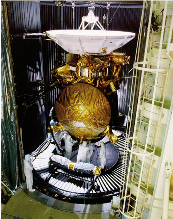
Figure 10.25. A picture of the NASA Cassini-Huygens spacecraft shown at the NASA Jet Propulsion Laboratory during vibration and thermal testing. Note that the NASA Cassini orbiter, with its large parabolic antenna provided by the Italian Space Agency, is in the back, and the ESA Huygens lander, being mounted in its circular gold Mylar covering, is in the foreground. NASA/GRIN/JPL digital image.
