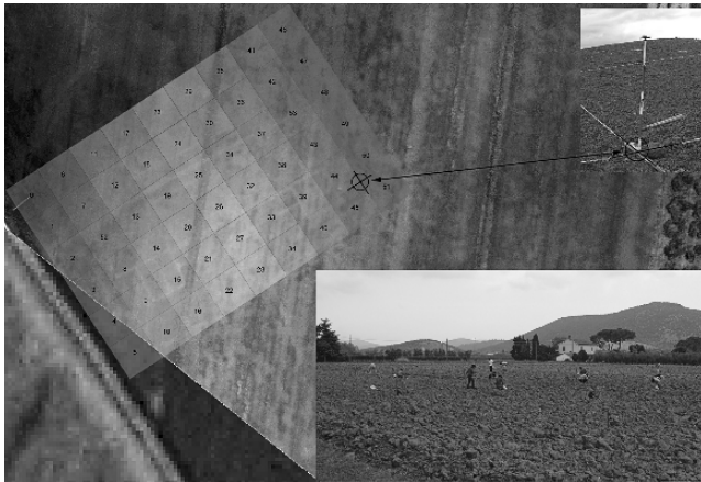
Figure 10. Collection of artifacts organized into “physical” predefined grids georeferenced through the differential GPS.
