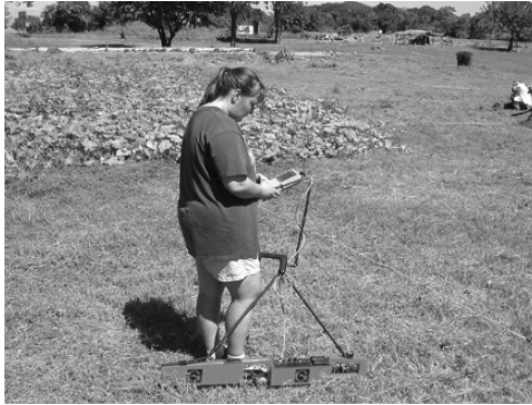
Figure 4. Jenny Bales operating the Geonics EM38B electrical conductivity meter at Ciudad Vieja, view to north. Photograph by Francisco Estrada-Belli.
