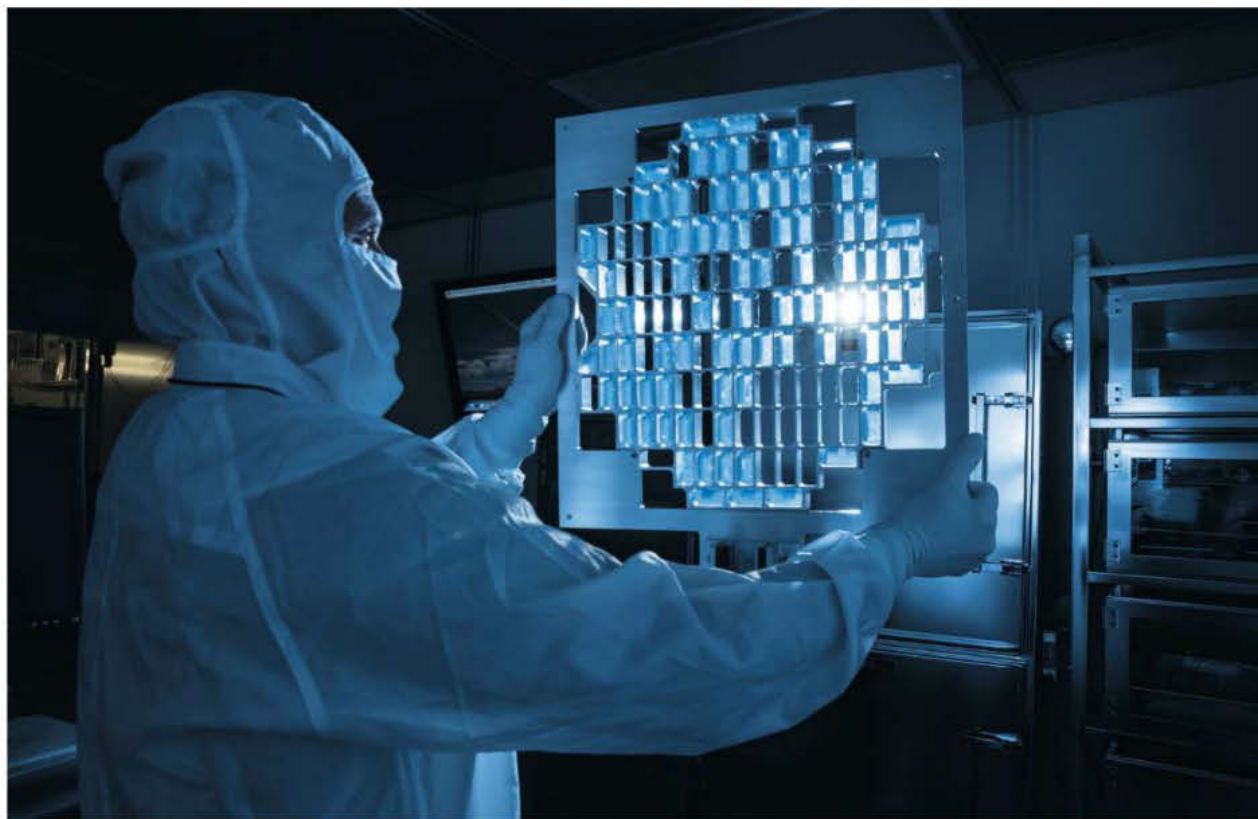
COMET DUST In a NASA clean room a scientist examines traps containing dust snared by the Stardust probe as it flew by the comet Wild 2. Each speck left a hair-size track (right) as it plunged into the puffy aerogel at more than 13,000 miles an hour.
