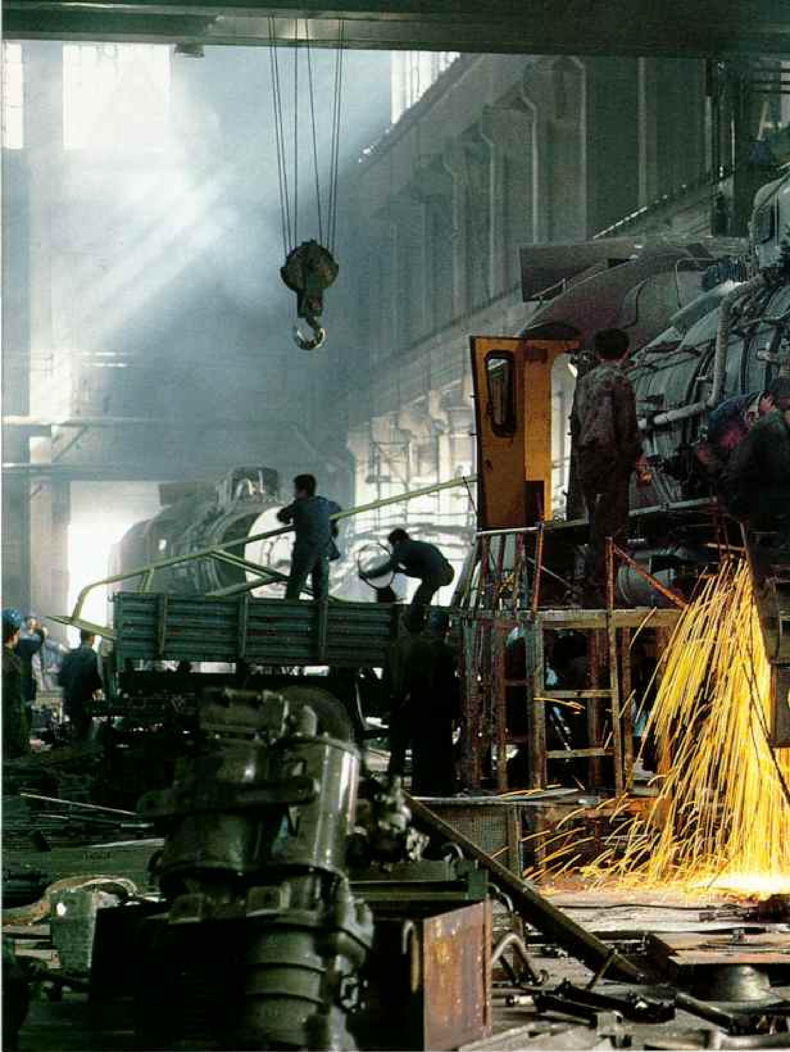
Orderly inferno reminiscent of the 19th century, the steam locomotive works at Datong labors to pull China into the 21st century. Welders join the boiler
