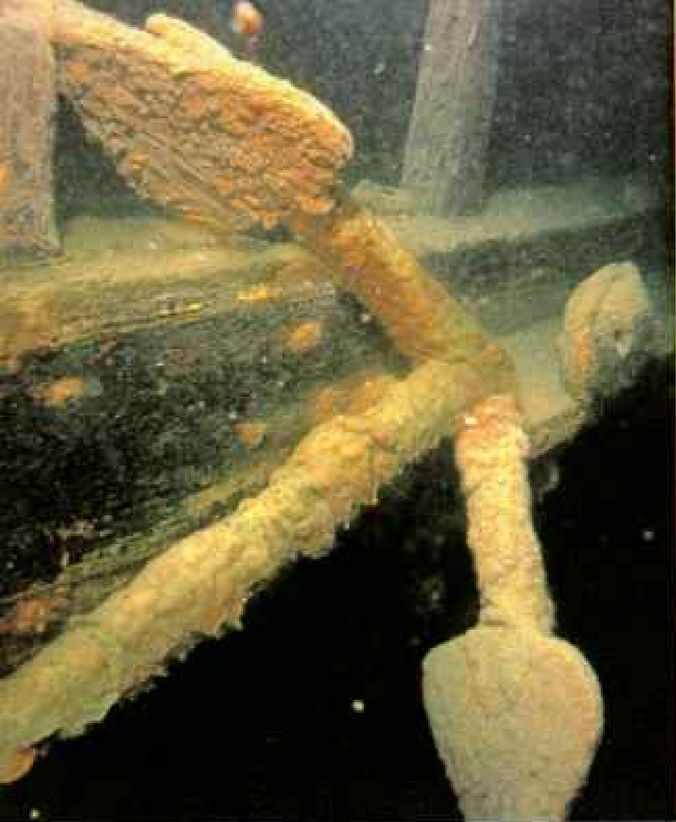
Hanging by a fluke, Hamilton's port anchor remains in its stowed position (left). The line that secured the anchor to a bitt next to the fluke has rotted away. Prior to stowage, the anchor was raised clear of the hull by passing its line through a cathead (below) that protrudes from the ship's bow.
