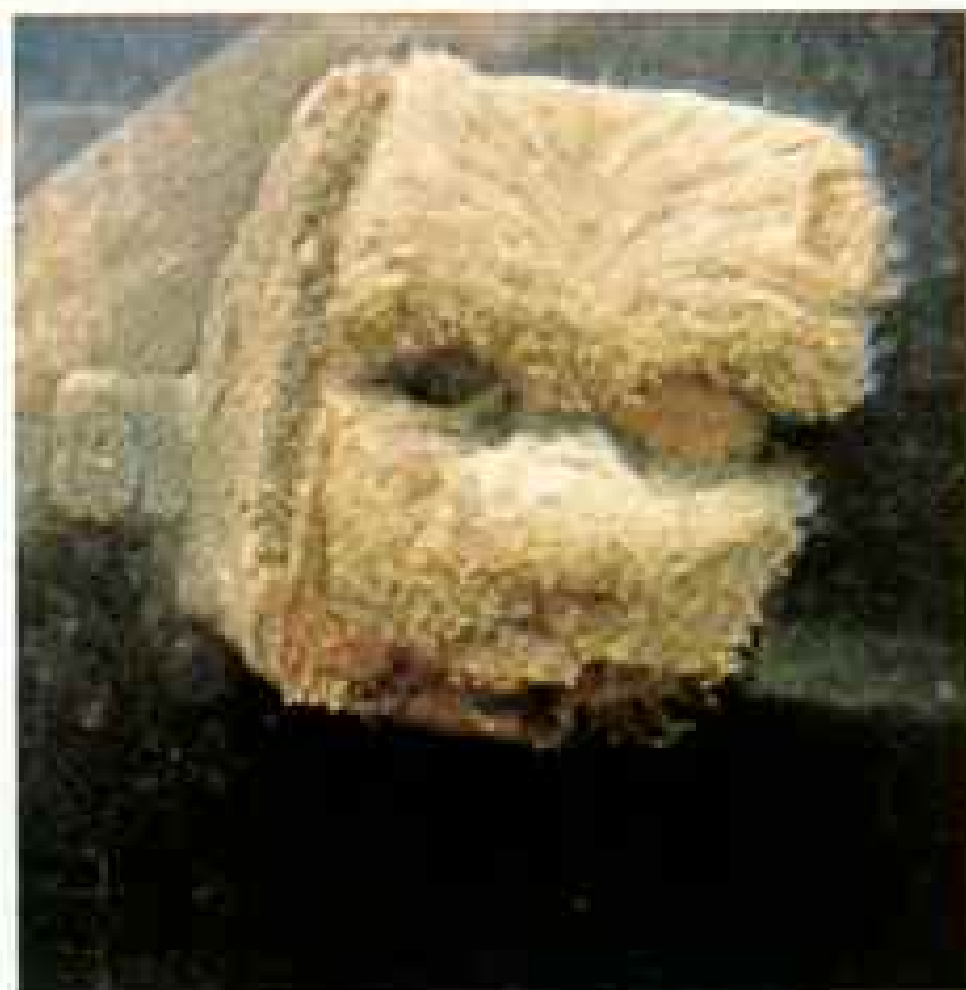
Hanging by a fluke, Hamilton's port anchor remains in its stowed position (left). The line that secured the anchor to a bitt next to the fluke has rotted away. Prior to stowage, the anchor was raised clear of the hull by passing its line through a cathead (below) that protrudes from the ship's bow.
