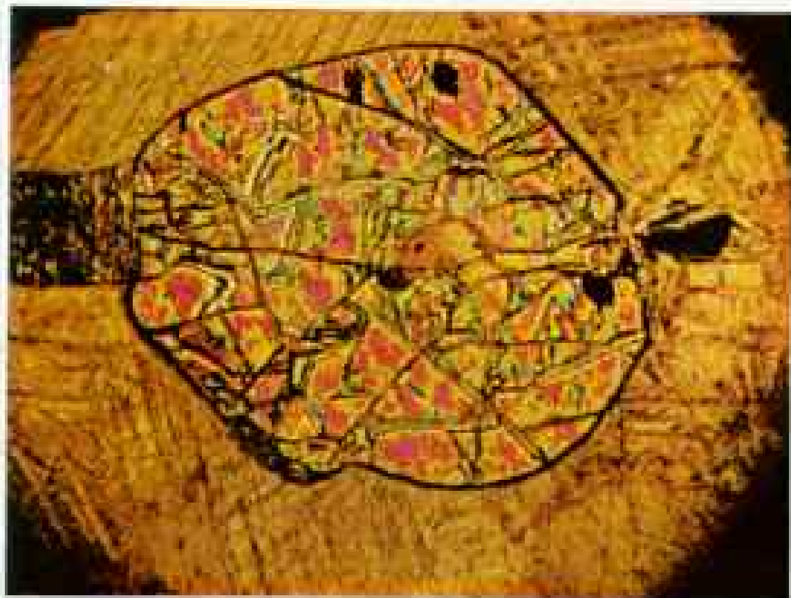
"Fossilized flounder" of olivine swims in a marble sea. The tiny crystal tells geologists that very high temperatures haked the marble from limestone.
