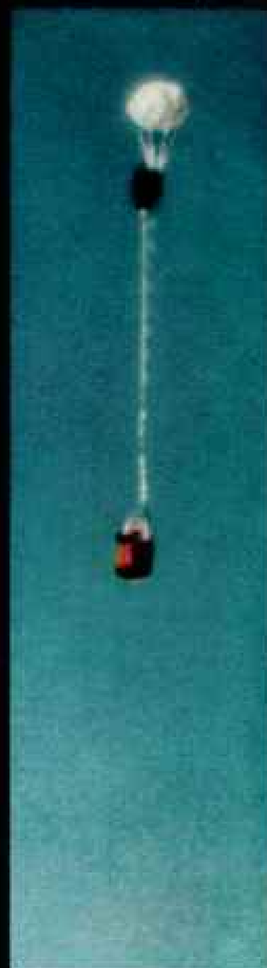
Drogue parachute drifts free after stabilizing descent and releasing the main canopy. Porthole camera caught chute and its canister falling to watery oblivion.
