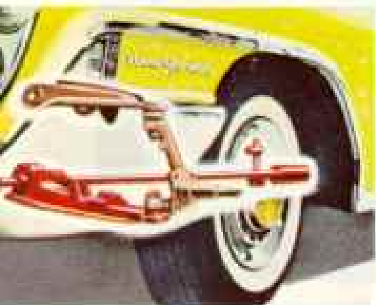
Smoothest-riding wagons on the road. Famous Torsion-Aire suspension gives you a "cloud smooth" ride even on rough roads. Standard equipment on all models.
