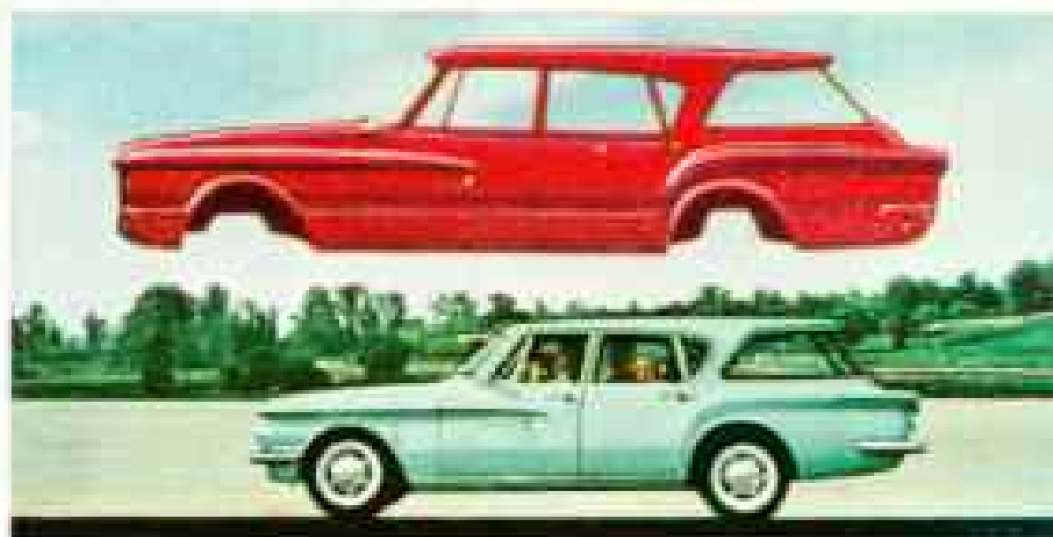
More room, less noise. Solid welded Unibody ends the major cause of squeaks and rattles, adds inches of space inside.
