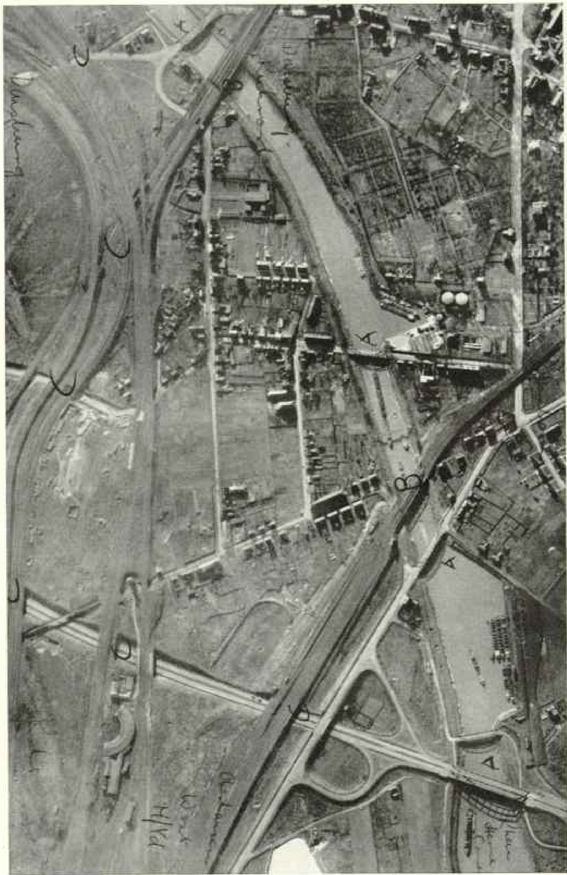
Shapes of Shadows Reveal the Types of Bridges in This German Transport Bottleneck Near Duisburg, on the Rhein-Herne Canal Letters, marked on picture by photo interpreters, indicate different kinds of bridges. "A's" are shown by shadows to be the joysting or arched type of suspension; "B's" are lattice girder; and "C's" plate girder. Heights of buildings, bridges, and trees can be estimated from their shadows.
