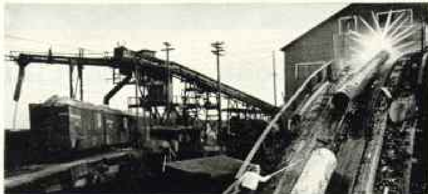
High pressure sprays clean off dirt and foreign matter as saw logs enter mill. This keeps saws sharp longer and improves quality of by-products.
