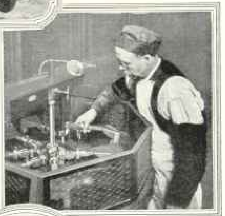
EVEN THE DIAMOND, after a long period of cutting hard rubber, needs to have its edge renewed. This grinding wheel, sprinkled with diamond dust, does the sharpening.
