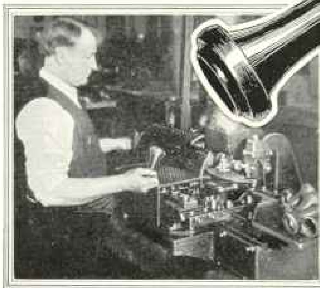
IN THE MACHINE pictured here a diamond is trimming away the rough edges, to prepare the receiver for your hand and ear.
