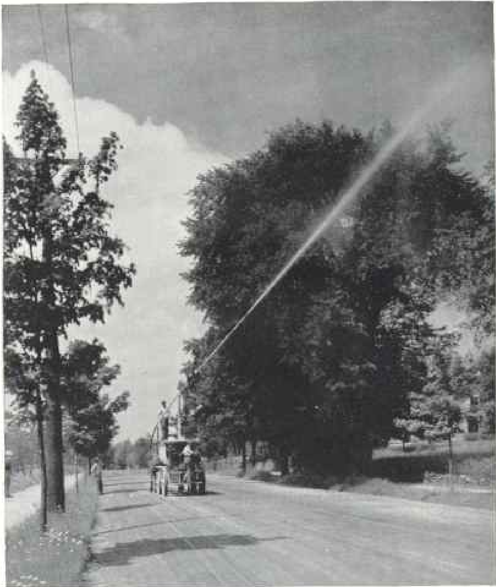
A HIGH-POWER SPRAYING APPARATUS TREATING A MASSACHUSETTS ROADSIDE WITH AN ARSENICAL WASH TO DESTROY GYPSY AND BROWN-TAIL MOTH CATERPILLARS.
