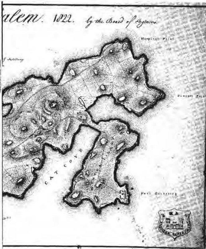
Figure 7.4. Comparative maps of Salem, Massachusetts, illustrating the contour ( left ) and hachure ( right ) methods of terrain representation by George Whistler and William McNeill (1822).
