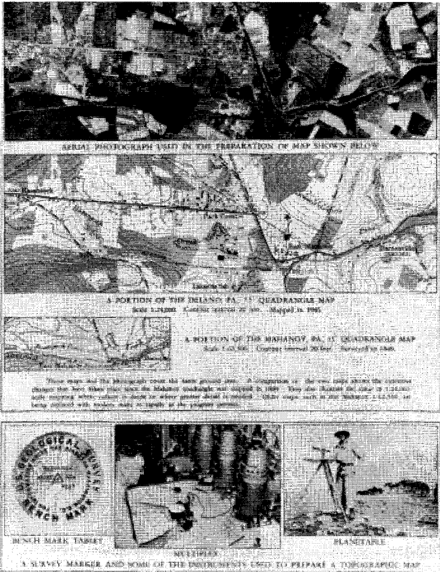
Figure 8.3. Layout showing the relationship between an aerial photo and a map, as well as maps of different scale and date. The lower panel illustrates a metal bench-mark tablet, a photogrammetrist, and a field surveyor at work. Prepared and published by the United States Geological Survey.
