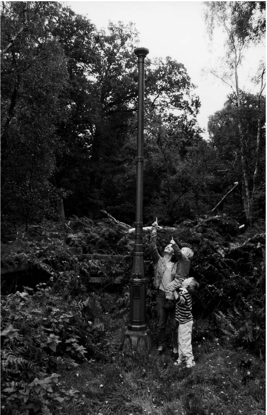
Figure 2.2 The Holme Fen Post near Peterborough, illustrating the substantial amount of peat shrinkage through drainage since 1848.
