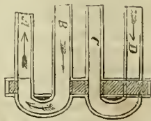
FIG. 3. CROSS SECTION OF WINDWAYS OF VALVE PLATE.
