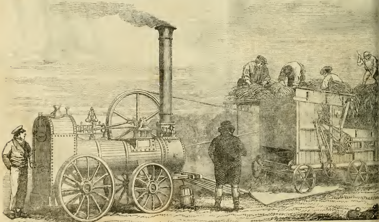
HORNBY'S PORTABLE STEAM-ENGINE AND THRESHING MACHINE.
