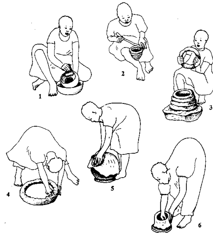
Fig. 6.3 African techniques of forming pots according to Olivier Gosselain: 1, pounding in a concave mold; 2, coiling (numerous variants); 3, superimposition and drawing of large rings; 4, drawing of a ring-shaped lump; 5, molding over a convex mold; 6, drawing of a lump.
