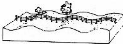
(D) Motion produced by a surface wave. Particles move in a circular path at the surface and diminish with depth.
