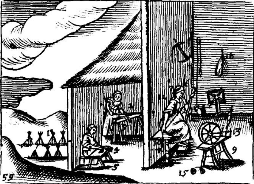
Figure 4.2 Spinning flax fibers into linen thread. The processes are roughly analogous to those for wool: on the left, women are cleaning and combing out the fibers, and on the right, a woman is using a drop spindle; next to her is a spinning wheel (Comenius 1887).
