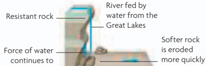
▲ The Niagara Falls were created where the Niagara River reached an escarpment capped by hard limestone. This was gradually eroded, exposing softer rock strata. Plunging water continues to erode the softer strata causing the falls to recede upstream.
