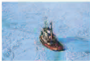
▲ Icebreakers are ships with specially strengthened hulls, designed to break a path through the ice. They are used to keep important routes open during the winter, when falling temperatures cause much of the Arctic Ocean to freeze over.
