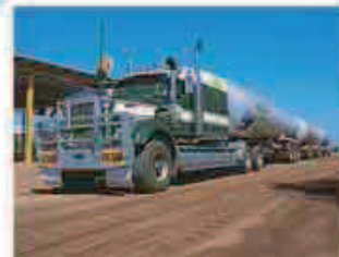
▲ Australia's vast interior is traversed by a limited number of vital roads, linking the major coastal cities to one another. Bulk freight crosses the country along these roads in huge articulated trucks known as "road trains."
