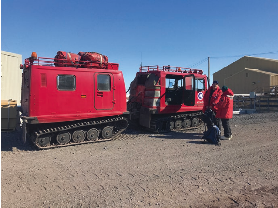
Fig. 1.12. The amphibious Haaglunds vehicles serve a variety of functions in the Antarctic environment (Photo by Rosaly Lopes)
