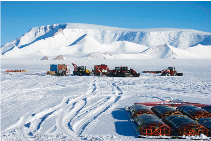
Fig. 1.13. Fuel is carried in giant bladders during the SPoT transports (USAP photo by Tim Thomas)
