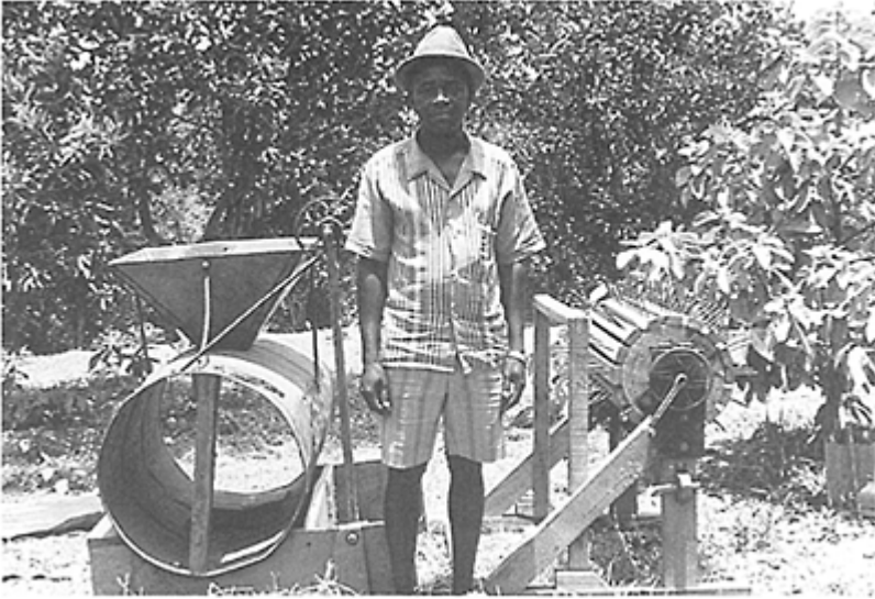
Plate 4.1 Enterprising farmer in Sierra Leone who has used his carpentry skills to make a threshing machine (right) and a winnowing machine (left)—good examples of intermediate technology, using indigenous skills and resources.
