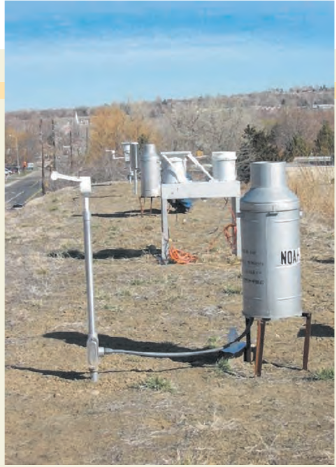
▲ Shown here are five different types of rain gauges installed in Arvada, Colorado. By placing the gauges next to one another, it is possible to compare how their precipitation measurements differ.
