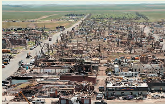
F5: 117–142 m/s (261–318 mph); strong frame houses lifted clear off foundation and disintegrated; steel-reinforced concrete structures badly damaged; trees completely debarked; automobile-sized projectiles thrown 100 yards or more
