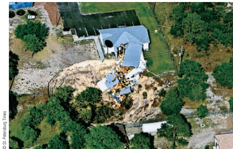
■ FIGURE 13.14 This large collapse sinkhole appeared in Winter Park, Florida, when a drought-induced lowering of the water table caused the surface to collapse into an underground cavern system.
