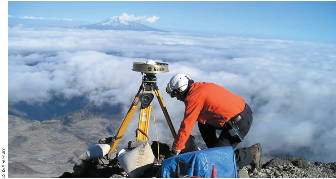
■ FIGURE 2.13 A scientist monitoring volcanoes in Washington state uses a professional GPS system to record a precise location by longitude, latitude, and elevation. This is the view from Mt. St. Helens, with another volcano, Mt. Adams, in the distance.
