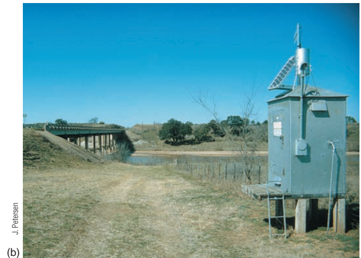
■ FIGURE 14.29 U.S. Geological Survey (USGS) stream gaging station. (a) As illustrated here, when river level rises or falls, so does the water in the lower part of the station, connected to the channel by intake pipes. A gaging float moves up and down with the water level, and this motion is measured and recorded. Gaging stations electronically beam flow data to a satellite that transfers the information to a receiving station. (b) Gaging stations are commonly located where highway bridges cross rivers or streams.
