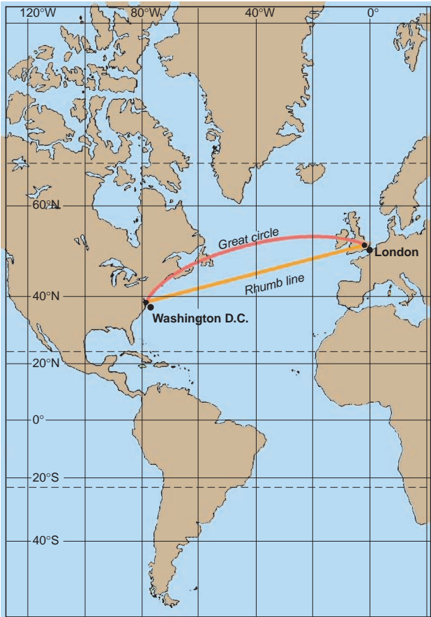
■ FIGURE 2.16 The Mercator projection was designed for navigation, but has often been misused as a general-purpose world map. Its most useful property is that lines of constant compass heading, called rhumb lines , are straight lines.
