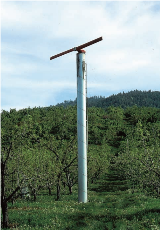
■ FIGURE 3.25 Propellers mix the air, breaking up inversions to protect these apple orchards in Washington from frost.
