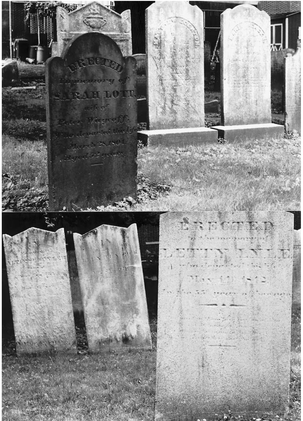
The grave marker at top is dated 1804, and the words are still clearly inscribed in the resistant stone. In contrast, the limestone grave marker from 1812 ( bottom ) is difficult to read because acid weathering has blurred the lettering. (Photographs courtesy of MACGES.)
