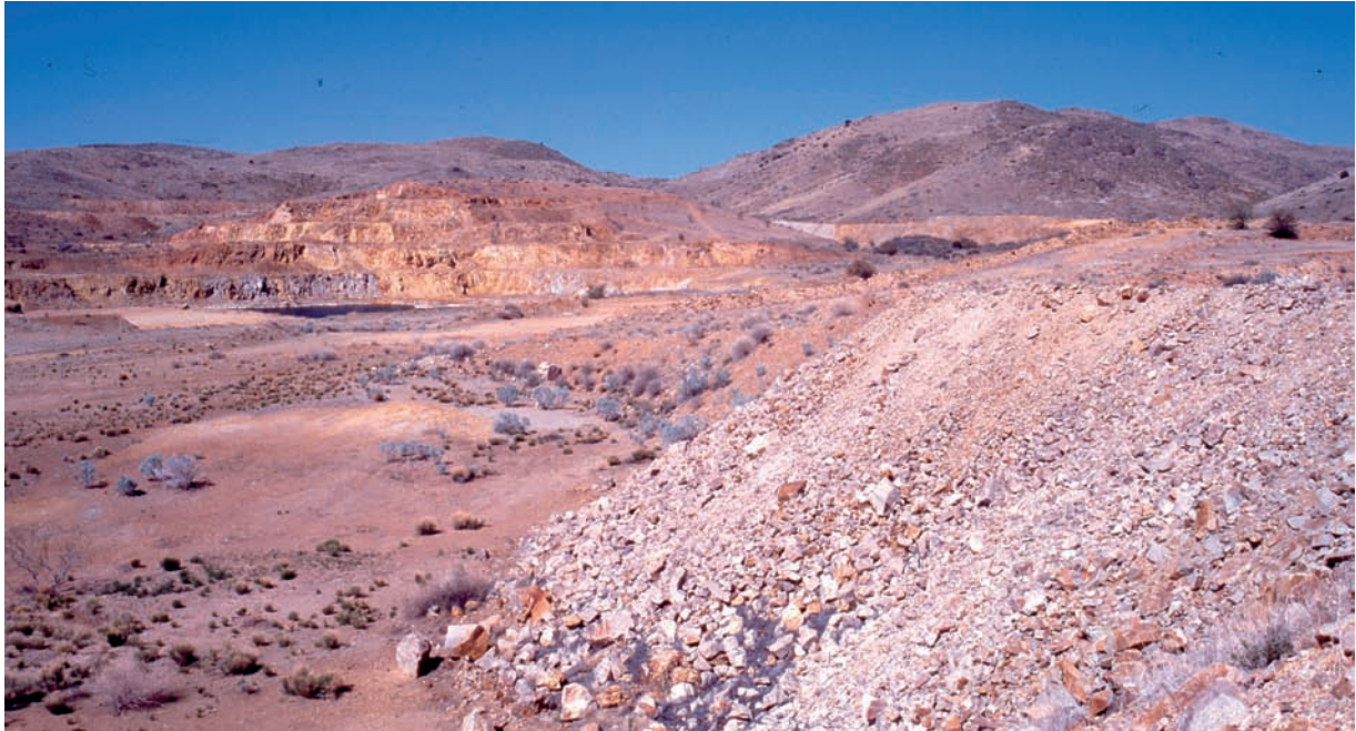
Figure 12.27 Unconfined spoil heaps of metal-rich material, Copper Flats copper mine, New Mexico, USA.
