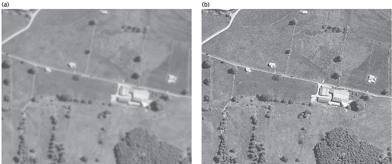
Figure 23.29 The image in Figure 23.27 is shown after applying (a) a low-pass filter which suppresses high-frequency variation in the image and (b) a high-pass filter which highlights the high-frequency variation in the image.
