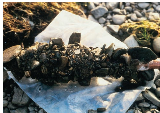
Figure 14.18 A vertical 'freeze core' of a gravel substrate. The core has been collected by inserting a tube into the sediment and then filling the tube with liquid nitrogen. This freezes the water around the tube and the nearby sediment thereby allowing it to be pulled out with the sediment intact for investigation. The core shows mixed grain sizes below the coarser 'armour' layer that is characteristically found at the surface.
