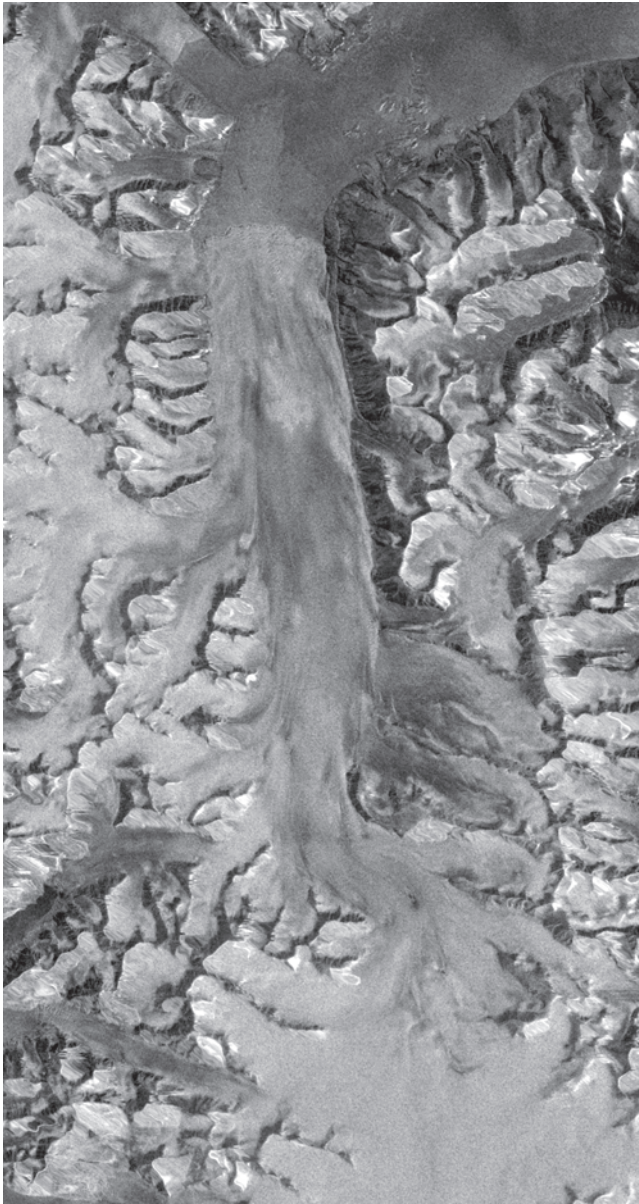
Figure 23.18 The radar image shown here shows Monacobreen (the Monaco Glacier) and surrounding mountains in north-west Svalbard, Norway. This image was captured in June 1995 by the ESA's Earth Resources Satellite (ERS). Notice the distortion in the mountain peaks due to the look angle of the radar instrument. North is up and the image is roughly 23 km across. (Source: image courtesy of Tavi Murray and Adrian Luckman)
