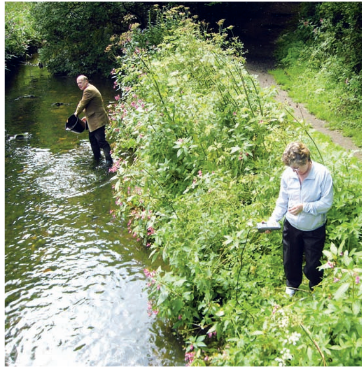
Figure 13.8 Measuring the concentration of sodium chloride in river water after it has been added upstream. The man in the background is adding a gulp injection from a bucket and the woman in the foreground is measuring the conductivity of the stream water using a conductivity probe and has a stopwatch to record the time. However, for the method to work effectively the two people should be much further apart for this size of river because the sodium chloride should be fully mixed with all of the stream water by the time it reaches the conductivity probe.
