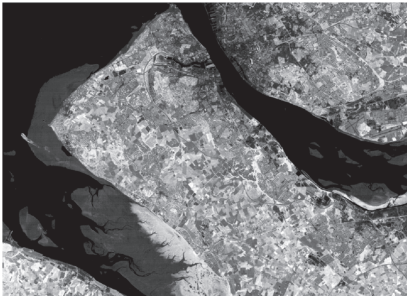
Figure 23.32 Landsat NDVI image which is generated using Landsat Bands 3 and 4 shown in Figure 23.31. Notice how clearly the city of Liverpool stands out against the parks and surrounding farmland as well as the brightness of the marshlands on the north shore of the Dee in the south-west corner of the image. (Source: image courtesy of MIMAS)
