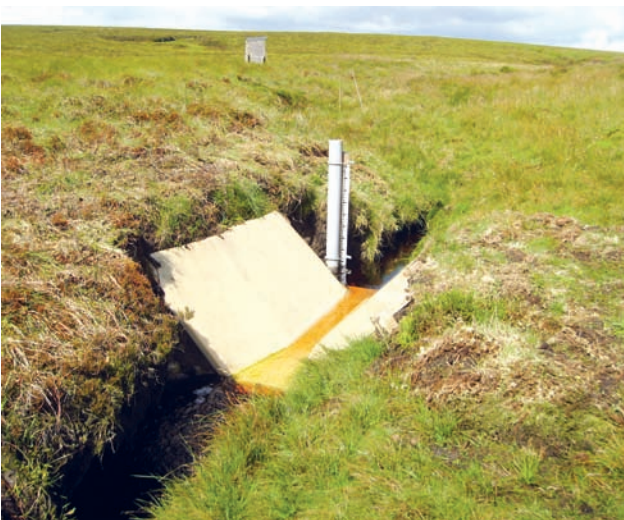
Figure 13.5 Gauging stations on the Tees catchment, northern England: (a) compound Crump weir, (b) V-notch weir, (c) flume-type weir.
