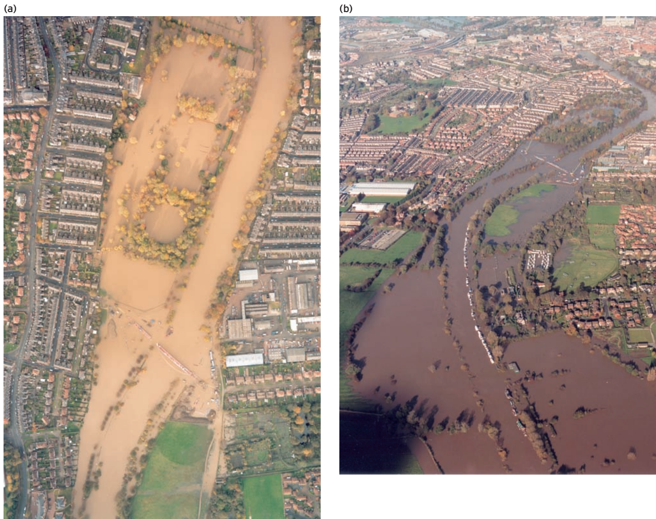
Figure 23.2 Vertical (a) and oblique (b) aerial photographs of the November 2000 flood of the River Ouse in the city of York, England. These images were used to map the extent of the flood waters for Britain’s Environment Agency. Notice how much more of the flood-plain is visible in the oblique image compared with the vertical image. (Source: photos © the UK Environment Agency)
