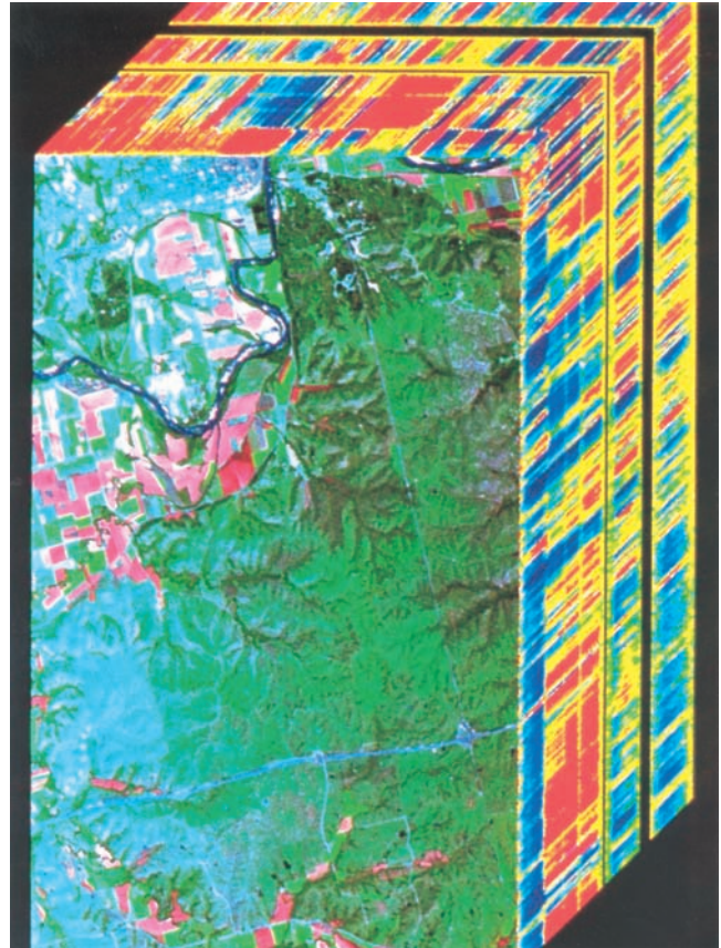
Figure 23.14 This image is an example of a hyperspectral image stack. The instrument used to capture the data was the Airborne Visible/Infrared Imaging Spectrometer (AVIRIS) which collects data in 224 bands of about 10 nm width between 0.40 and 2.45 \mu\text{m} . This particular image was captured over Konza Prairie, Kansas, in late August. (Source: from Lillesand and Kiefer, 2000)
