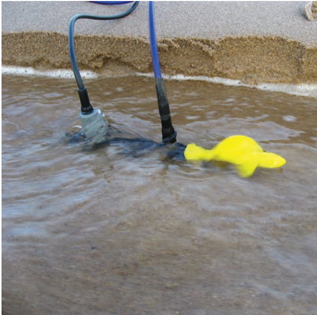
Figure 1.7 Investigating flow in a sandy stream. The presence of the flow meter in the water causes changes to the water movement that the flow meter is trying to measure.
