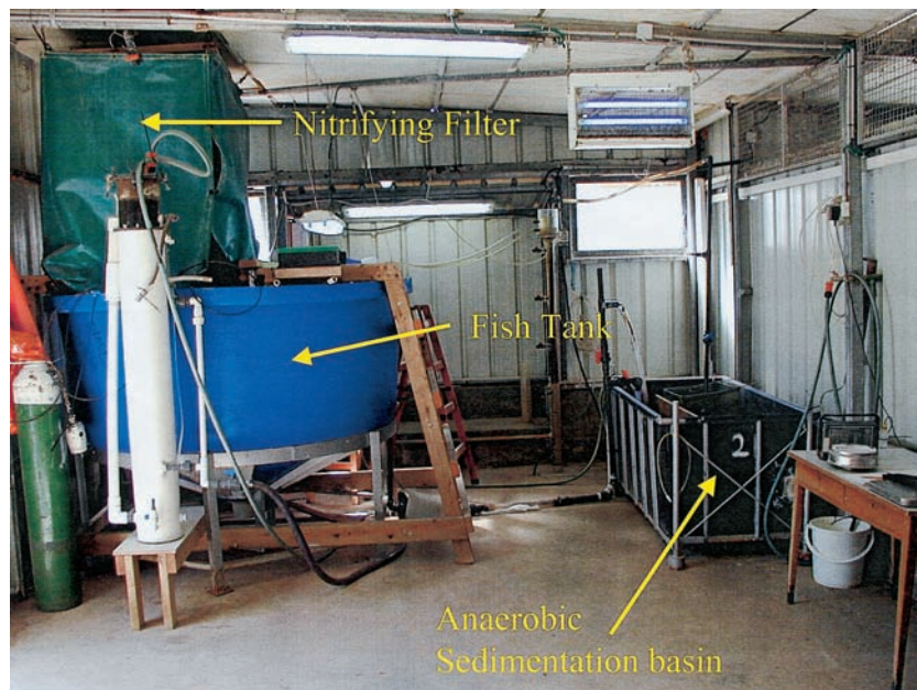
Figure 3.21 This pilot mariculture system uses bacterial biofilters to clean the waste nutrients from the water and enable the system to operate with no waste water discharge at all.
