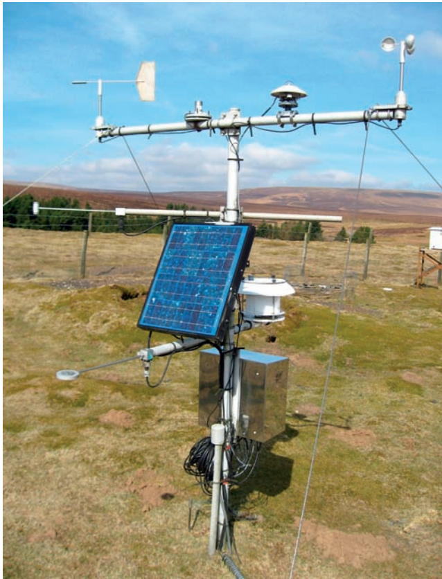
Figure 5.1 An automatic weather station. The blue solar panel is used to charge the battery supply.
